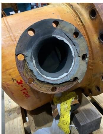
Before Belzona 2111 repair
