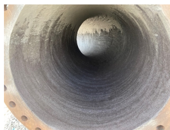
Dredge pipe after bottom half coated with Belzona 1814 working outward from center. Pipe was flipped over to complete job while making for easier application.
