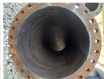
Dredge completely coated with Belzona 1814.
