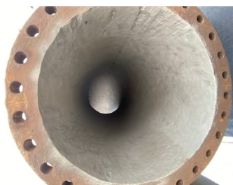
Dredge pipe after being blasted by application team.
