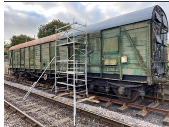
Belzona 3111 is applied to the roofing area
