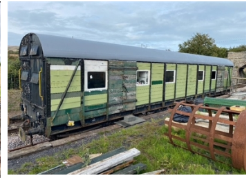
Completed application, restoring integrity to roof
