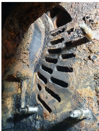
Heavily corroded sealing face.
