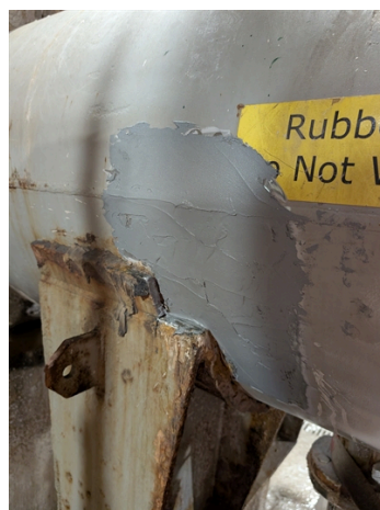
Rebuild with Belzona 1161 with 9341 mesh
