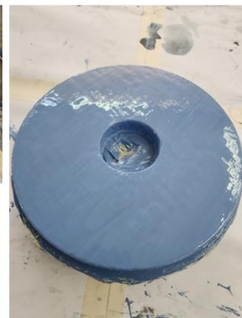
An impellor suffered corrosion from prolonged exposure to water
