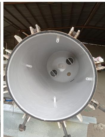
Existing lining failed and started to show sign of corrosion
