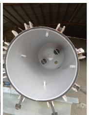
Existing lining failed and started Old lining was removed before Coating during process to show sign of corrosion the repair
