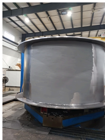
After rebuilding with Belzona 1121
