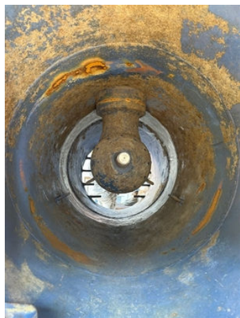
Bow thruster tunnel suffering from pitting due to electrolysis.
