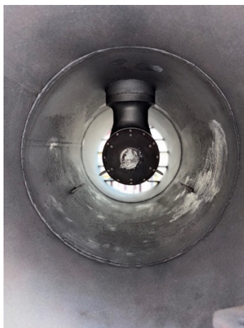
Bow thruster tunnel blasted to required SSPC-SP10.
