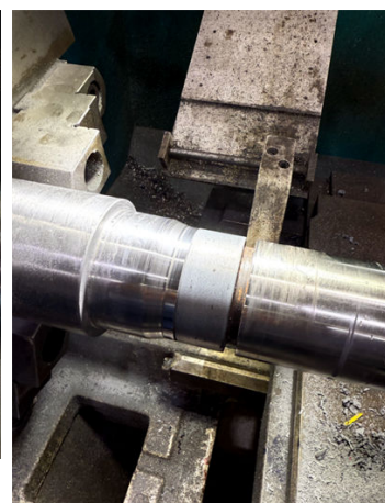
Final result after machining. The shaft was rebuilt with Belzona 1161 and restored to its original diameter and smooth finish.
