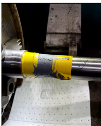
Application of Belzona 1161 (Super UW-Metal) using a plastic former to rebuild the eroded area and restore original shaft dimensions.
