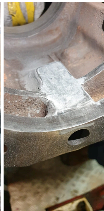
Belzona 1311 applied & then machined flat with the surrounding metal
