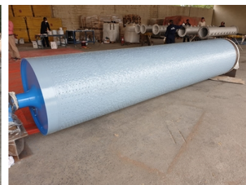
Dryer roller after the application of Belzona 1511 (Super HT-Metal) and Belzona 1391T to restore metal loss
