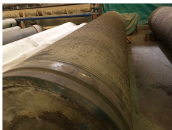
Corroded dryer roller caused by chemical washing, high temperature and humidity
