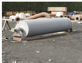
Surface preparation via abrasive grit blasting
