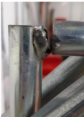
Typical failed weld on a transportation cage
