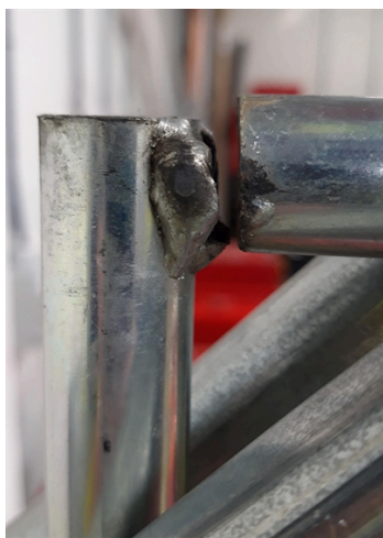
Typical failed weld on a transportation cage
