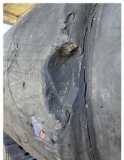
Large tears and gouges reduced Damaged areas were cut back the efficacy of the Fender and caused ropes to become caught and then prepared with a
