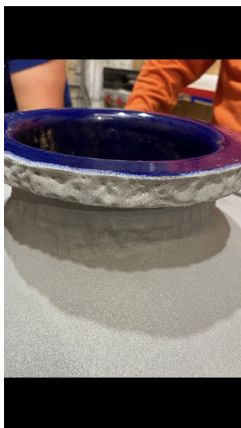
After abrasive blasting the externals, SSPC-SP10
