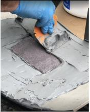
Then we applied Belzona 1111 for the adhesion of the plate along with Belzona 1812 tot he center of the plates for wear resistance.
