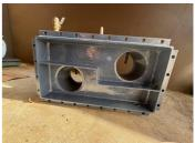
exchanger access covers is shown prior to repair. The surfaces exhibit severe corrosion, material loss, and deterioration around the tube sheet, resulting in leaks and unsafe operating conditions.
