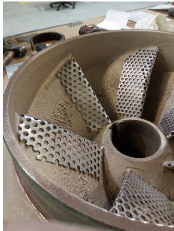
Giving this impeller back its leading edges
