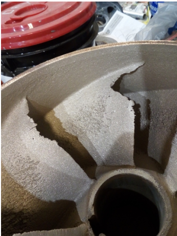
Notice leading edge of impeller blades
