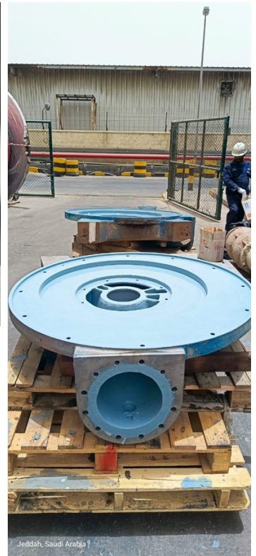
Pump cover coated with Belzona 1391T
