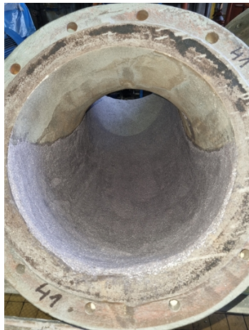
Pipe elbow after application of Belzona 1812.
