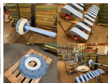
The fully repaired and coated turbine components.
