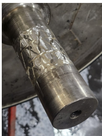
Shaft are prepped using a hand grinder.
