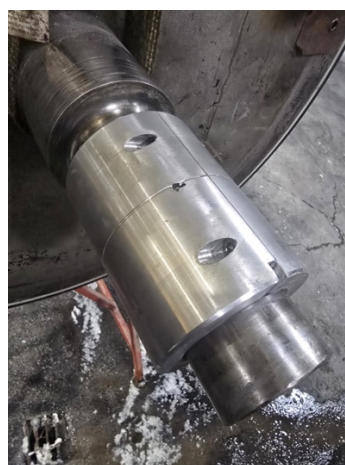
Customer made former in place with the Belzona 1111.
