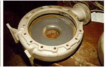
The finished casing ready for re-assembly
