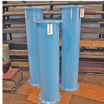
Other pump parts coated inside out with Belzona 5812DW
