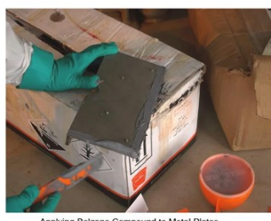
Applying Belzona Compound to Metal Plates
