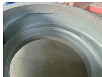
Repair detail with Belzona 1812 and 1391 products
