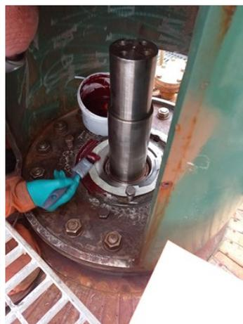
Area prepared & wetted out with Belzona 4331
