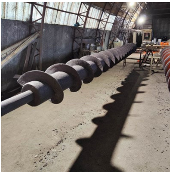
Belzona 1812 was applied on the screw flights and shaft.
