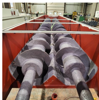
Close up of the completed application of Belzona 1812
