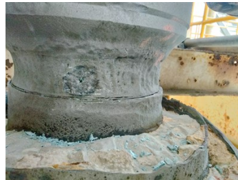
Surface after grit blasting.
