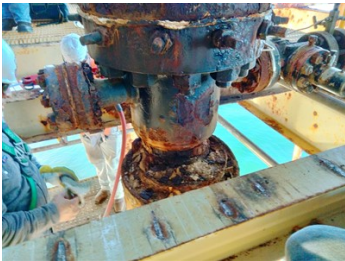
Original condition of the leaking wellhead.
