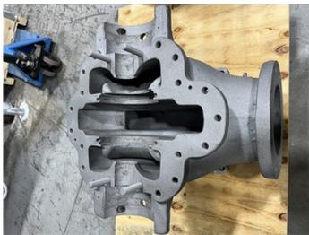
Pump after being sandblasted/prepared.
