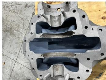
Second Coat of Belzona 1321 (blue).
