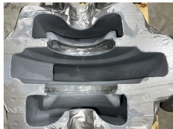
First coat of Belzona 1321 (grey).
