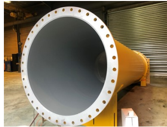
Finished internal & external lining application using Belzona 5811.
