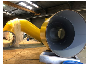
Finished internal & external lining application using Belzona 5811.
