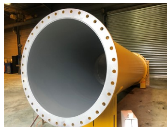
Finished internal & external lining application using Belzona 5811.
