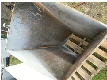
New chute pre-coating
