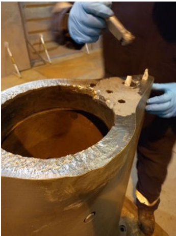
Surface preparation carried out & Belzona 1111 applied
