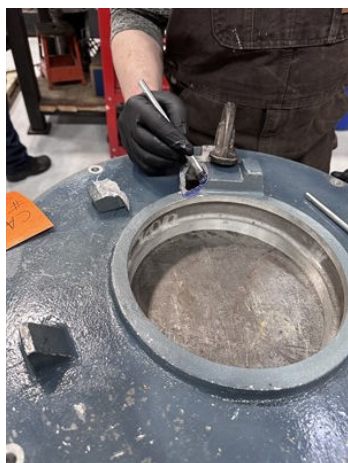
Applying 7311 to Cover
