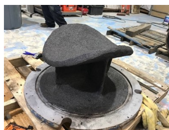
Finished coat of Belzona 1814
