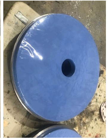
Super smooth rebuilt and coating of Belzona 1341 to the pump plate
