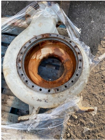
Casing before coating showing wear from service
