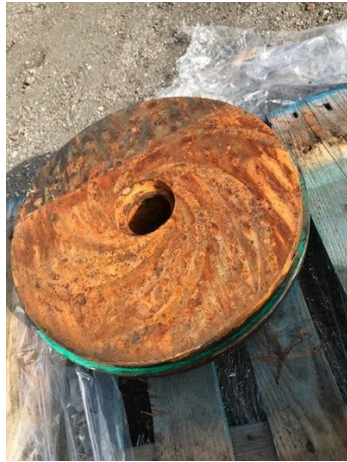
Pump plate before showing service wear
