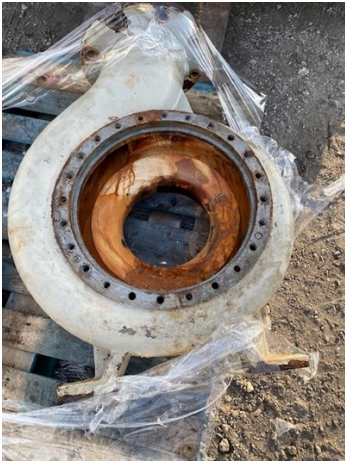
Casing before coating showing wear from service
