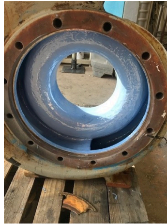
Freshly rebuilt and coated pump casing
