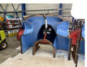
Damage caused by erosion-cavitation leading to a substrate loss greater than 5mm.
