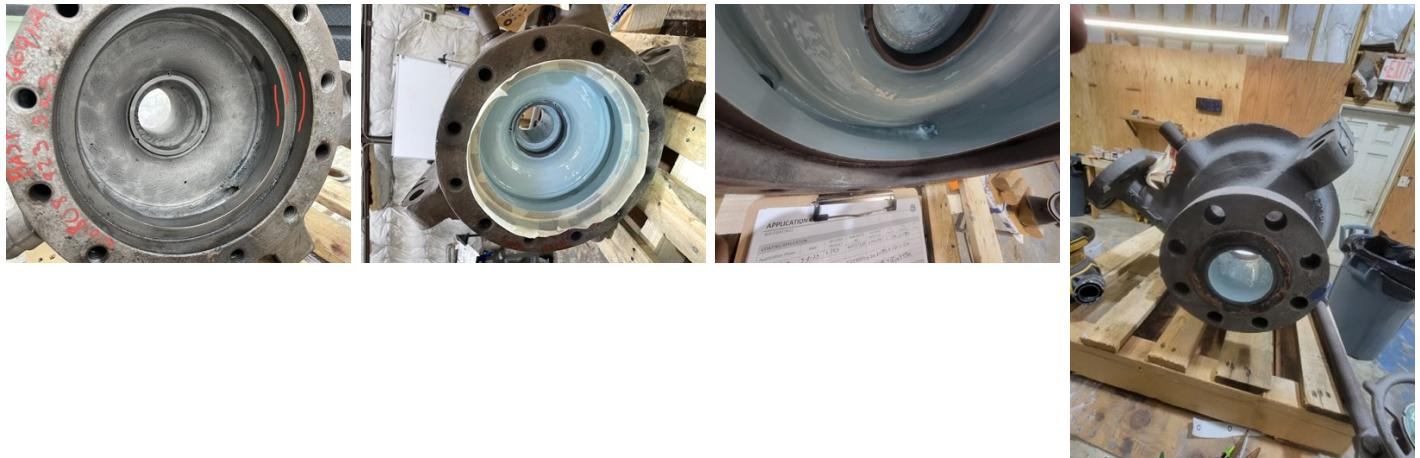
Pump internals after it was abrasive blasted. Two small holes shown.
