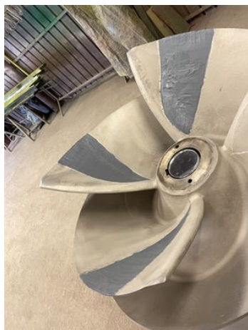
Rebuilding the damaged surface
