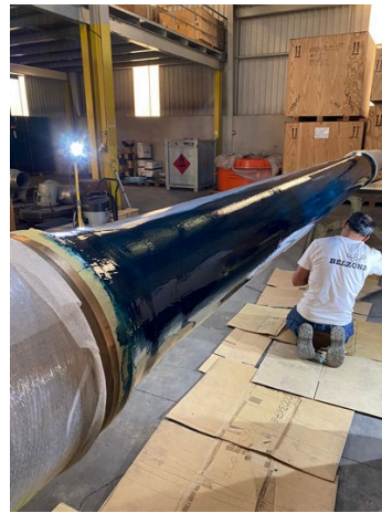
3.) 1st coat of Belzona 2141 being applied
