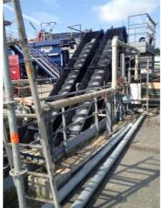
Screw during the Belzona 1341 Screw & trough once application.
