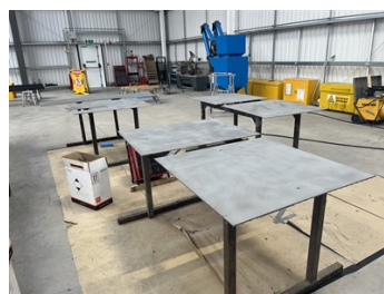
Cover plates prepared as per Belzona 4351 (Magma CR5) IFU
