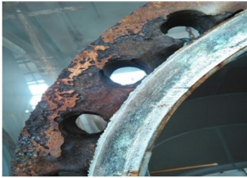
View of damage to the flange
