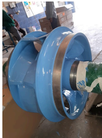
Fully coated impeller for protection
