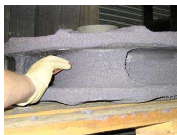
Impeller rebuild &amp; lining
