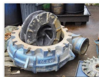
The lining condition after 18 months of service
