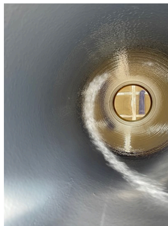
Internal coating of Belzona 5821 on pipe
