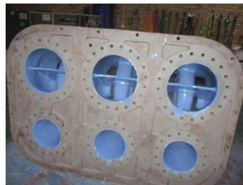
Split casing pump repaired and protected with Belzona
