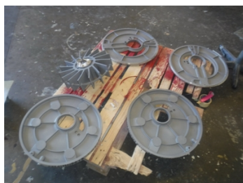
After sand blasting
