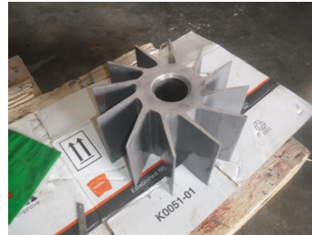
The impeller rebuilt with Belzona 4301
