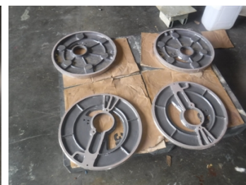
The suction and discharge disks after coating with Belzona 4311
