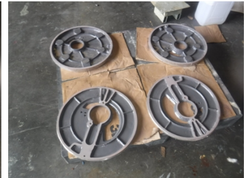
The suction and discharge disks after coating with Belzona 4311
