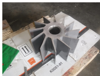
The impeller rebuilt with Belzona 4301
