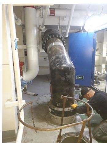
The steel pipe affected by scrubber exhausted emissions
