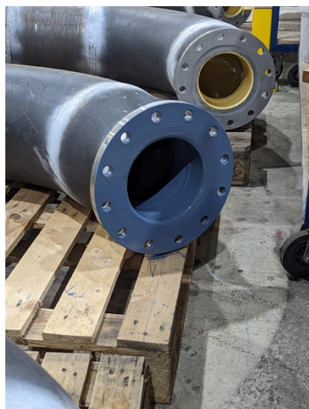
Internals coated with Belzona 5821
